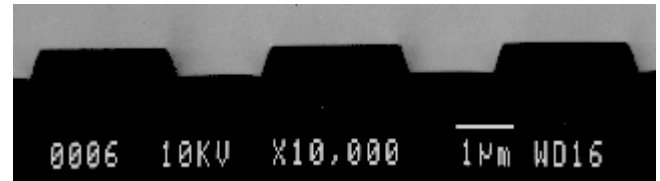
Figure 1. Cross-sectional view of 4 \mu\text{m} period Si relief grating. We estimate the structure as: period = 3.96 \mu\text{m} , top linewidth = 2.2 \mu\text{m} , depth = 0.5 \mu\text{m} , and wall angle = 73°.
