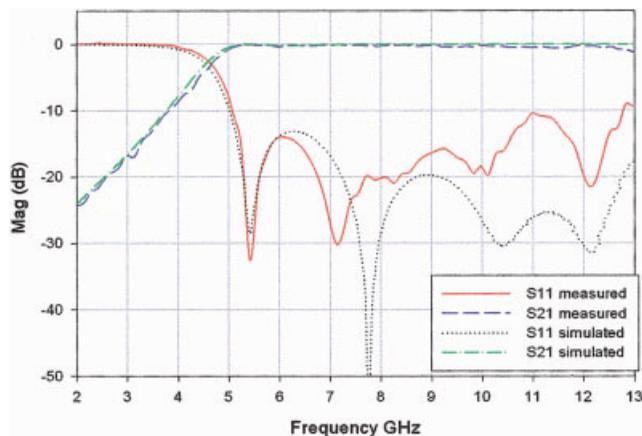
**Figure 3** Response of the suspended coaxial transmission line. [Color figure can be viewed in the online issue, which is available at [www.interscience.wiley.com](http://www.interscience.wiley.com).]
