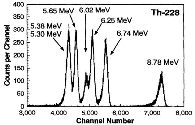
FIG. 6. Alpha particle differential pulse height spectrum from  $^{228}\text{Th}$  taken with a 100  $\mu\text{m}$  bulk GaAs detector. The detector was irradiated in vacuum from the front contact (Schottky contact).
