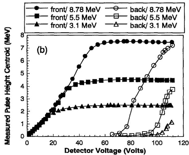
FIG. 5. Comparison of front and back irradiation with alpha particles for a 100- $\mu\text{m}$ -thick bulk GaAs detector. Shown are (a) the numerically calculated pulse height responses and (b) the measured pulse height responses. The alpha particle energies are 3.1, 5.5, and 8.78 MeV.  $\mathcal{E}_c$  is  $7.0 \times 10^3$  V/cm and  $\alpha$  is 15. The pulse height response is shown in terms of energy (MeV) measured from the detector.
