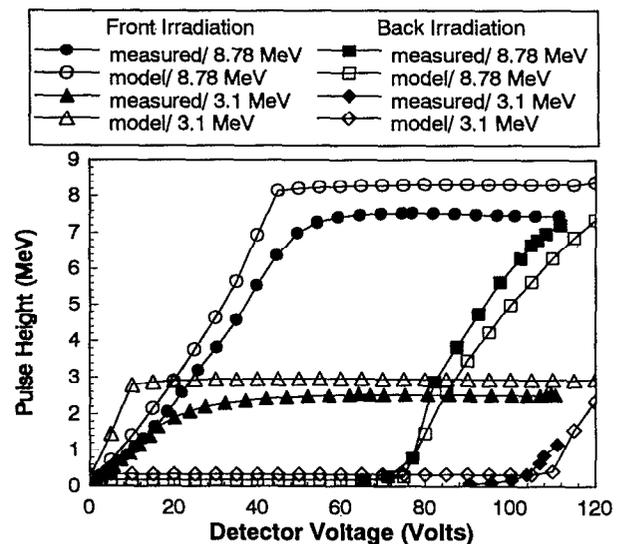
FIG. 7. Overlay comparison between modeled and measured pulse height curves for a 100- $\mu\text{m}$ -thick bulk GaAs detector. Shown are the curves for 3.1 and 8.78 MeV alpha particles where the pulse height response is shown in terms of MeV.  $\mathcal{E}_c$  is  $7.0 \times 10^3$  V/cm and  $\alpha$  is 15 for the modeled pulse height curves.
