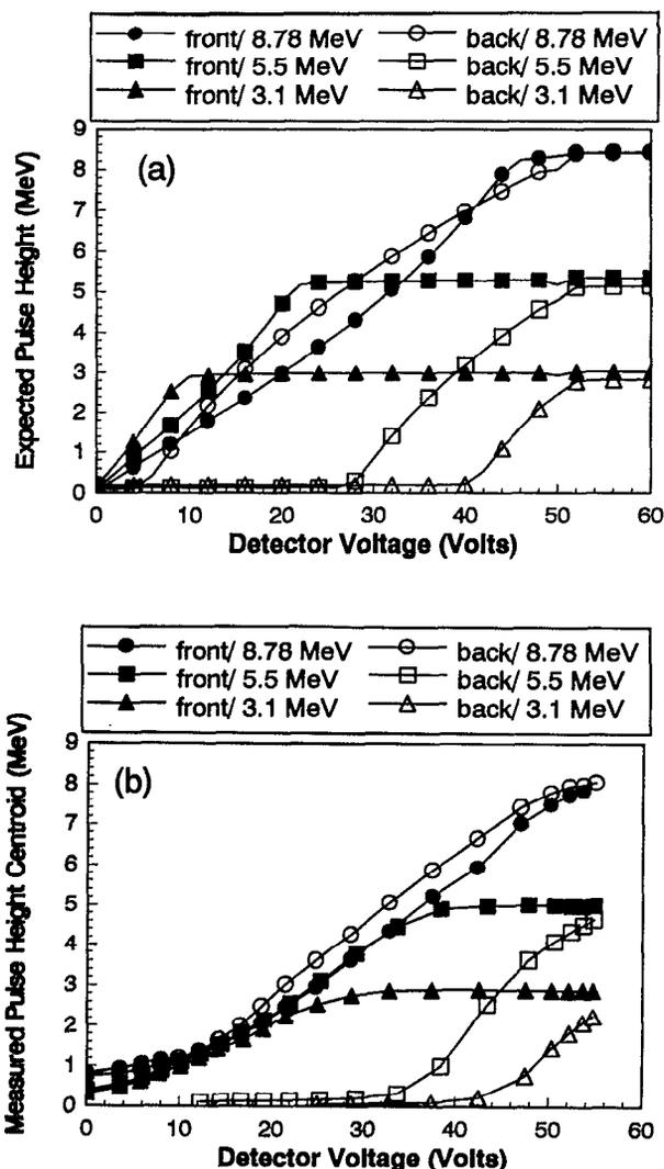
FIG. 4. Comparison of front and back irradiation with alpha particles for a 45- $\mu\text{m}$ -thick bulk GaAs detector. Shown are (a) the numerically calculated pulse height responses and (b) the measured pulse height responses. The alpha particle energies are 3.1, 5.5, and 8.78 MeV.  $\zeta_c$  is  $7.0 \times 10^3$  V/cm and  $\alpha$  is 15. The pulse height response is shown in terms of energy (MeV) measured from the detector.
