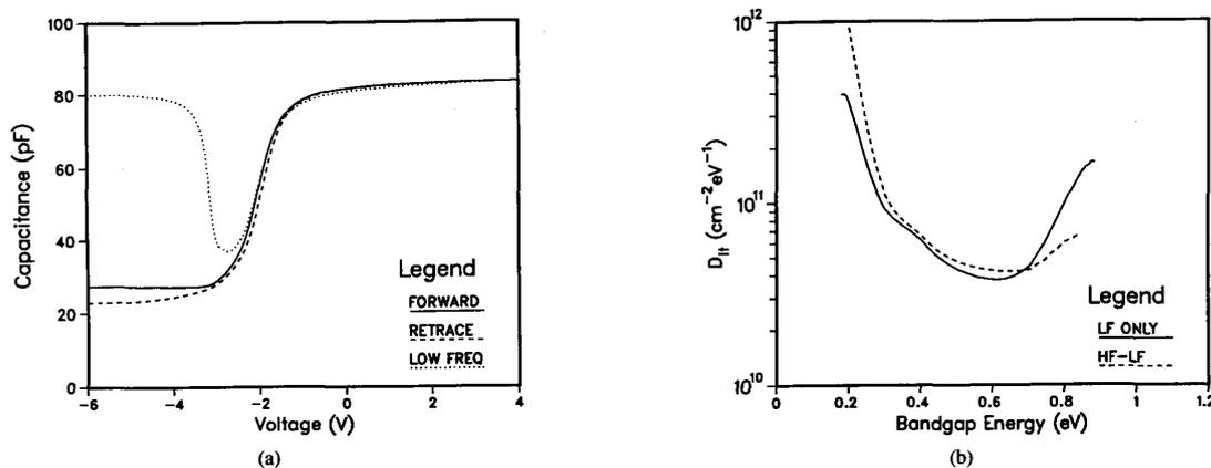
Fig. 1. 100-Å  $\text{SiO}_2$  deposited at 300°C, hydrogen plasma during temperature ramp, followed by 900 Å deposited at 350°C: (a) high- and low-frequency  $CV$  curves and (b) interface trap density.
